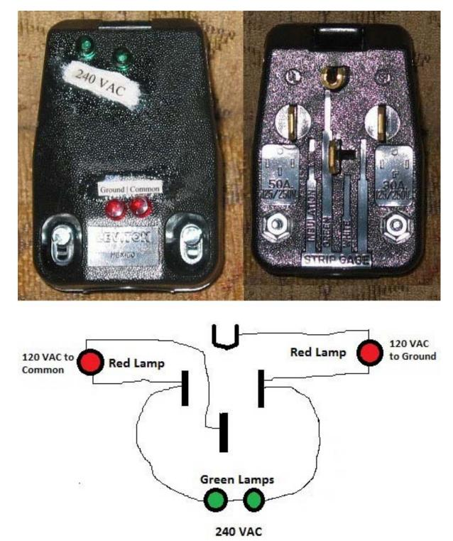
I used a 240 VAC 50 Amp plug from Ace Hardware and two Red & two Green 120 VAC indicator lamps from Radio Shack to build this test unit.
